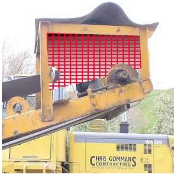
Suggested Guarding for left side of conveyor drive drum
