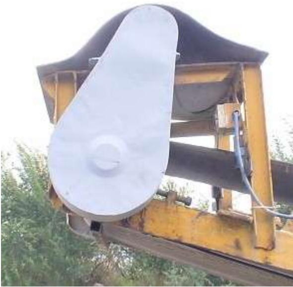
Suggested Guarding for right side of conveyor drive drum
