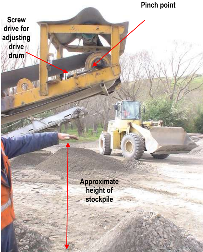
Conveyor and drive drum
