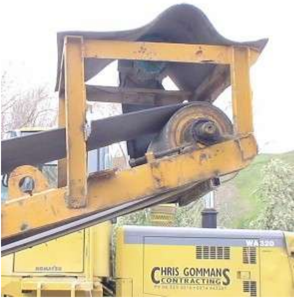
Suggested Guarding for left side of conveyor drive drum
