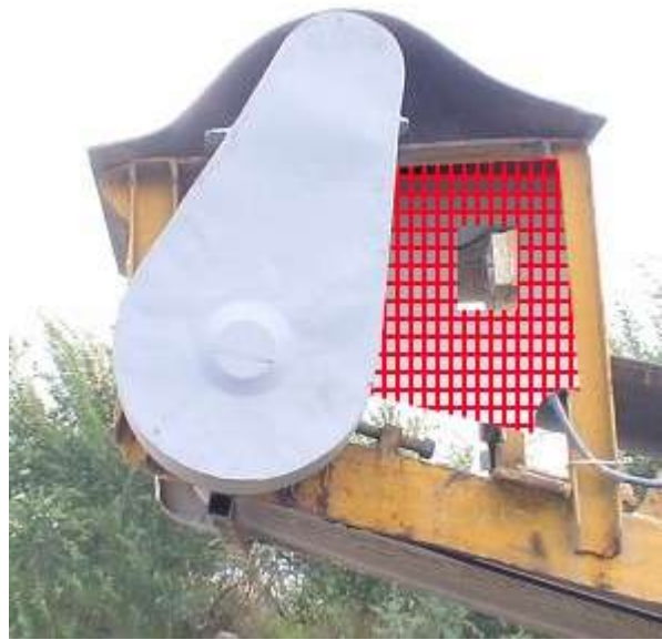
Suggested Guarding for right side of conveyor drive drum
